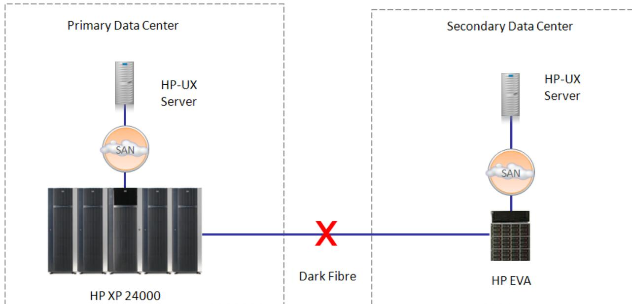
The first step was the creation of the physical and logical paths between the XP24000 and the EVA for use by External Storage. A vdisk was then created on the EVA and presented to the XP24000. Next, the volume was discovered on the XP24000 via External Storage and paired via Continuous Access Synchronous with an internal XP24000 volume using the RAID manager utility.
